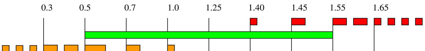
**B:** rEvo 1.0 pulse code: when PPO2 = 1.0, only the green LED is ON continuously. For every 0.1 bar above 1.0, the red LED will pulse once. (up to 1.5 bar). For every 0.1 bar below 1.0, the orange LED will pulse once.
