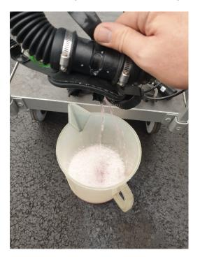
9: when drained, give the unit 3 rinsing cycles with fresh water until all traces of the cleaning solutions have disappeared (foam, pink color). Remove the breathing hose, rinse with fresh water, and remove water from the hose by pressing the hose together in a vertical position
