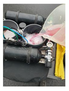
7: after the 10 minutes, move the closed DSV / BOV sideways so it acts as a pump to move the solution to the exhale scrubber compartment. Leave it another 10 minutes
