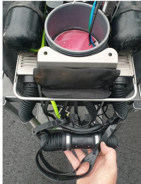
8: after 10 minutes in the top compartment, drain the unit using the DSV/BOV and by unscrewing the exhale breathing hose connector (housing side). Keep the Virkon solution for canister disinfecting
