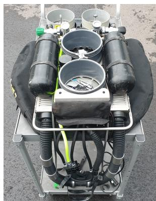
3: Remove the sensor tray from the bottom scrubber housing, if you disconnect by the wet connectors, make sure to use blanking plugs to protect the wet connectors (R563 A / B) . This ensures that the oxygen sensor tray (sensors and connectors) stay clear of the disinfectant solution.
