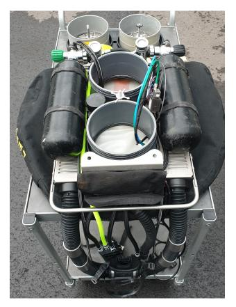
5: Open both tanks valves, a pressurized gas system is a good way to prevent water ingress in the gas supply system
