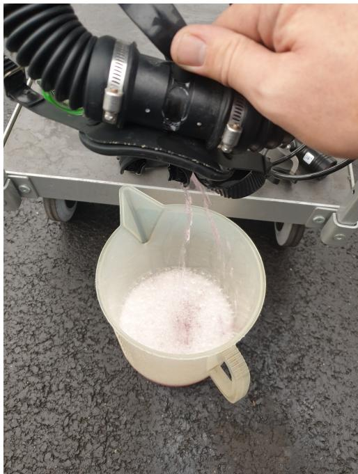
9: when drained, give the unit 3 rinsing cycles with fresh water until all traces of the cleaning solutions have disappeared (foam, pink color). Remove the breathing hose, rinse with fresh water, and remove water from the hose by pressing the hose together in a vertical position
