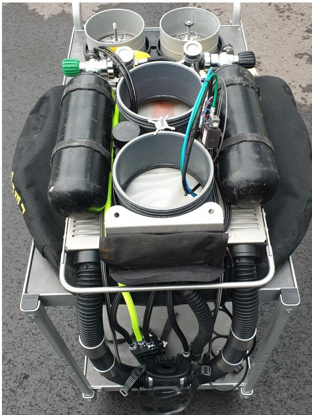
5: Open both tanks valves, a pressurized gas system is a good way to prevent water ingress in the gas supply system
