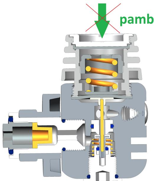
At surface the IP is set at 10 bar absolute, and using the same orifice, at surface we have the same volume flow of 1l/min. (+/-1.43gr/min)
