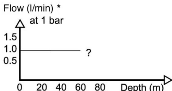
And this is what we want when we have oxygen flowing into a rebreather: we inject an amount of oxygen into the breathing bag, so that it just compensates for the basic oxygen consumption of our body (metabolic consumption) when we are at rest, or moving very slowly. And since our metabolic consumption does not change with depth, we don't want the oxygen mass flow into the breathing bag change when we descent or ascent: we want it to stay constant.
