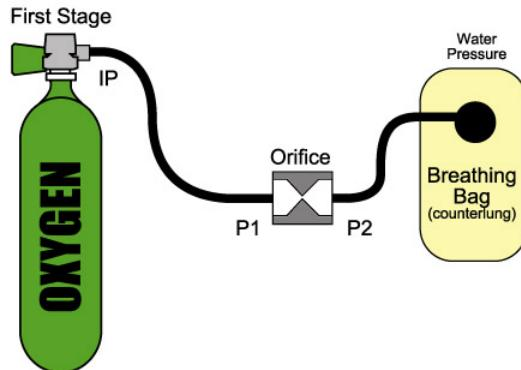
Suppose we choose the diameter of the orifice this way, that at surface, with the IP, or  $p_1$ , set at 10 bars, we have a flow of 1 l/min (measured at the surface!!), so  $\pm 1.43$  grams/min.  $p_1$  is 10 bars, the outlet pressure ( $p_2$ ) is 1 bar (at surface), so  $P_1$  is more than twice  $P_2$ , we have 'sonic speed', so we reach maximum volume flow.
