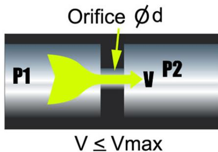
So, when the conditions to reach maximum or sonic speed are achieved, whatever you do, increasing the pressure at the entrance of the hole, decreasing, or even vacuuming on the exit side of the hole, the speed of the gas travelling through the hole will not increase anymore, but stay constant at  $V_{max}$ .
