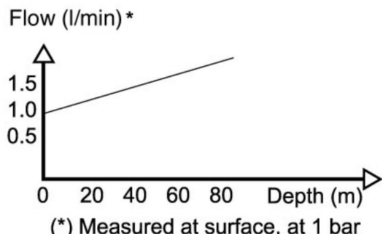
We notice the deeper we go, using our system with a standard scuba regulator (that has a compensated first stage) connected to the oxygen tank, the mass flow of oxygen (and so the
