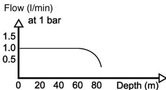
And while we go deeper, 70m, 80m ... the pressure in the water  $p_2$  will increase and come closer to  $p_1$  (the IP), the velocity of the gas will keep dropping and so will the mass flow, until we reach 90m. At that point the pressure in the water equals the intermediate pressure (both 10 bar), there is no pressure difference over the orifice anymore, so no gas will flow through it, the mass flow has dropped to zero.
