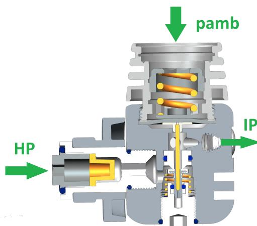
so we can say that with a compensated first stage, the IP (intermediate pressure) is depending on the ambient pressure.
